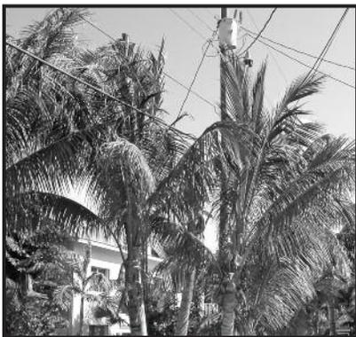
*Example of the wrong tree in the wrong place...* These palms were planted directly under power lines. Over time, as they matured they posed a threat to electric and other utility's service. Because palm trees cannot be topped or pruned away from power lines they must be removed to maintain reliable electric service.
